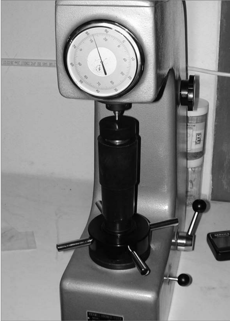
Figure 1 The resulting impression is measured and the hardness can be read on the scale
